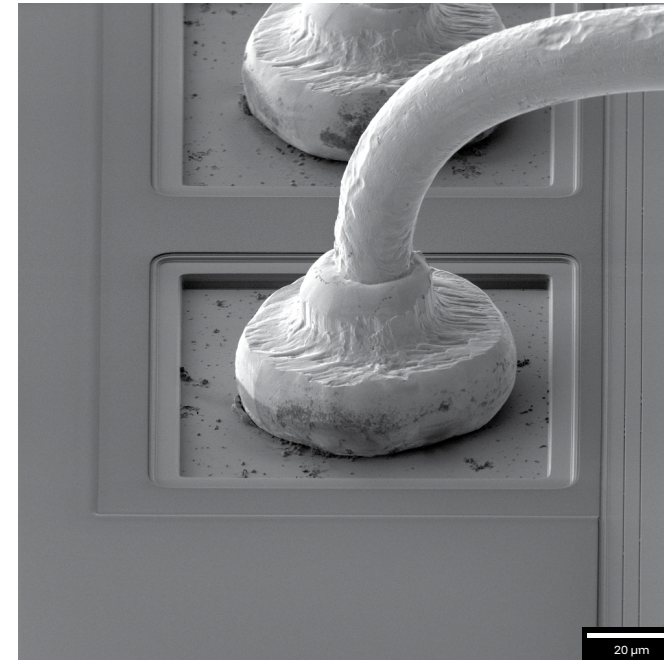
(both) Au ball bond imaging at 2 keV, Everhart-Thornley SE detector.
