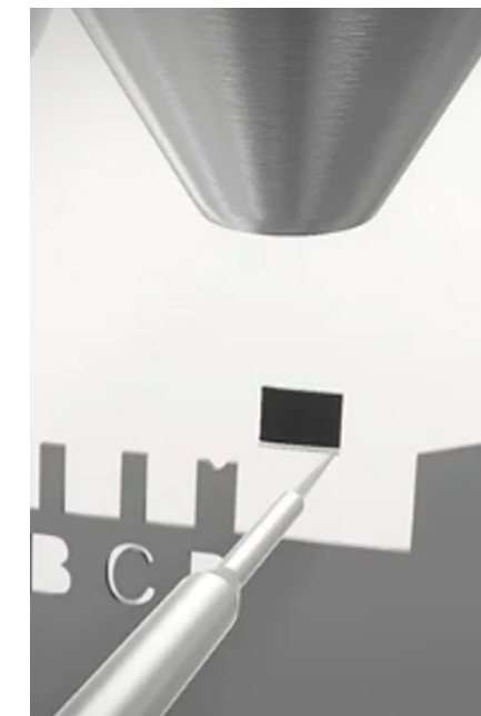
Unique, patented position of the nanomanipulator below the FIB enables preparation of planar, inverted, and other TEM sample geometries with ease.
