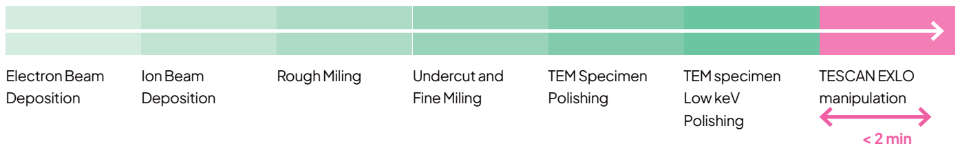
Figure 1: Workflow comparison between fully automated in situ lift-out and TESCAN's automated sample preparation combined with TESCAN EXLO™ ex situ transfer. While in situ lift-out offers a fully automated and user-friendly workflow, transferring the lift-out step outside the FIB-SEM with TESCAN EXLO™ reduces the total time per sample by up to 20%. This results in a higher number of specimens prepared per day and a lower cost per specimen, making it an efficient alternative for high-throughput and cost-driven environments.
